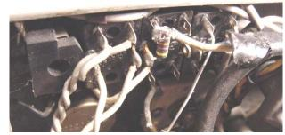
usually be cured by spraying the switch contacts with 'Servisol' or DeOxit' contact cleaner. Multi-pole/sectional 'wafer' switches are notorious for such faults as they are often carrying very low signal levels and their contacts are exposed to all manner of potential contaminants/oxidants – oil residues from lubrication attempts,
