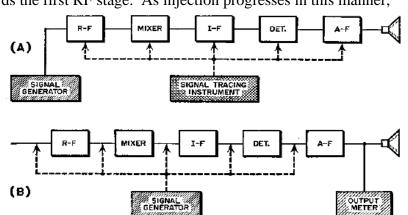
Dynamic troubleshooting analysis may be divided into signal-tracing and signal-injection methods. (A) illustrates the signal-tracing system and (B) shows the signal-injection system.
