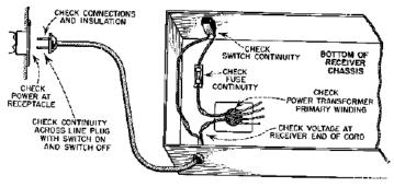
either side of the fuseholder(s), then on either side of the mains switch, then the transformer primary. If the appropriate AC voltage is not present on any of these locations, identify the cause and correct (suspects are a blown fuse, broken wire,
