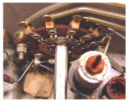
in response. If it does, the problem can usually be cured by spraying inside the control with 'Servisol' or DeOxit' contact cleaner and rapidly 'working' the control several times: if it does not, replace the control. If it is an RF or IF gain control however, be sure to use a wirewound replacement part. If it is the AF gain control, use a log-law carbon track part.
